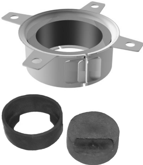
Firepro B310 FWD Pipe Collar Floor Waste System is designed specifically for situations where there is a requirement to meet the specifications of AS4072.1-2005 Section 4.6.2 on 100mm ID uPVC & PE pipes penetrating concrete floor slabs. The FWD Disc and Puck are not required to meet Section 4.6.1.
