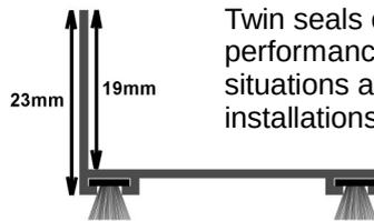
Twin seals offer superior sealing performance, particularly in under door situations and to sides of sliding door installations. DLB & DLF Seals come with slotted holder for simple installation or adjustment.
