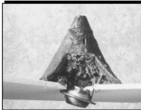
In a fire situation, the cover expands internally to fill the available space with fire-resistant insulating material.
